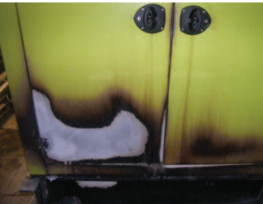
CONTAMINATED RAG STARTS FIRE
